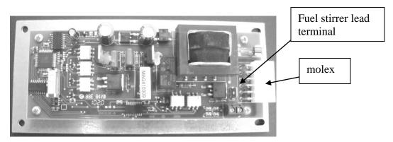
5 Fuel Stirrer motor black wire from control panel to one black lead double white lead
