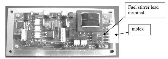
black wire from control panel to one black lead double white lead to black lead
