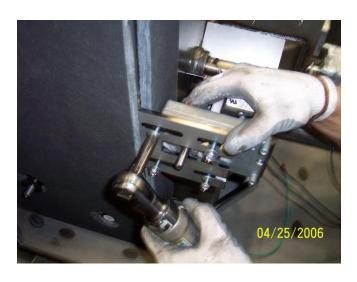
Position fuel stirrer motor and tighten loosely. Keep screws loose until chain is in place using hardware listed above.
