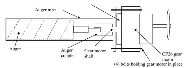
It is very important that the CF26 gear motor assembly is installed properly so that the alignment is straight with the auger shaft.
