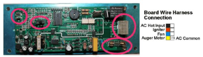
8 amp 120 Volt Fuse Fast-Blow Cartridge Fuse
