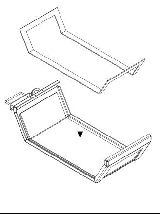
8. Place the brackets that secure the glass assembly in place and secure with nuts. Do not overtighten the nuts as you make break off the stud welds.
