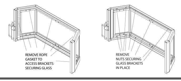
4. Once all the brackets are removed, you can disassemble and remove the glass, gaskets and vertical glass corner pieces and clean them off. Once they are cleaned, re-install the vertical glass corner pieces as shown.
