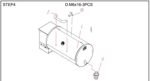
4. Use M6x16 screws and shrapnel to install the upper cover handle on the barbecue barrel; Use M6x16 screws to install the limit baffle on the grill barrel and hang the oil receiving barrel on the grill barrel.
