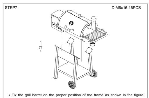
above, and use M6x16 screws to lock it from the outside of the grill barrel.
