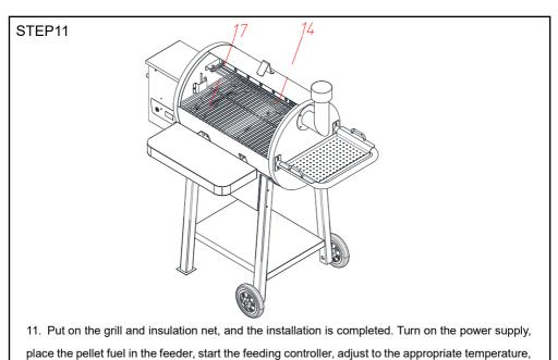
and smoke the food when the temperature of the cylinder rises to the set temperature.
