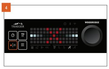
If your probe has been successfully disconnected, you will hear an audible "disconnected" tone and the display will show this animation. The probe icon in the probe menu bar will flash and then turn off.
