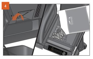
Once the hopper is empty, close the door and tighten the knob. Refill the hopper with a different flavor of TRAEGER HARDWOOD PELLETS.
