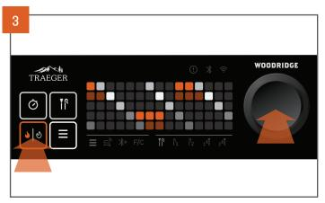
When the grill is in idle (display showing: - - - F), press and hold both the ignite/shutdown button and the selection dial. The auger will begin to move and the screen will display the auger moving animation.
