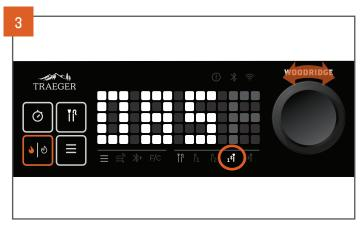
From the probe menu, use the selection dial to cycle through and highlight any of your probes that are currently connected and active. You will see the icon light up in the probe menu bar, and the current probe temperature will be displayed.
