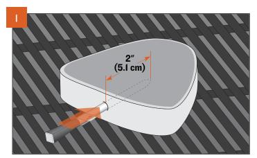
Insert the probe up to the notch, into the thickest part of the protein—avoid touching any bones or particularly fatty portions of the protein. The probe needs to be in the protein at least two inches (5.1 cm). This probe may not be suitable if you cannot insert the probe two inches (5.1 cm) into the thickest part of the protein. After your probe has been inserted, load your food onto the preheated grill.
