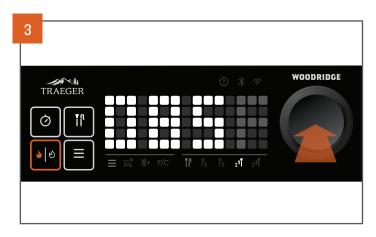
When the desired probe is highlighted in the probe menu bar beneath the dot matrix display (probe I shown above) and the current probe temperature is displayed, press and hold the selection dial for three seconds.
