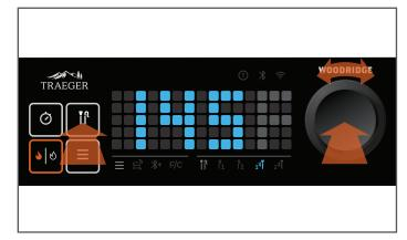
**CANCELING:** If you'd like to cancel a probe goal alarm, simply tap the probe button and use the selection dial to navigate to the desired probe (in this example, Bluetooth® probe I). Then press and hold the selection dial for three seconds. After pressing and holding the selection dial, the goal alarm will be canceled and the numbers will revert back to white and display the current probe temperature reading.
