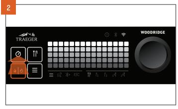
Press and hold the timer button for three seconds to clear the timer.
