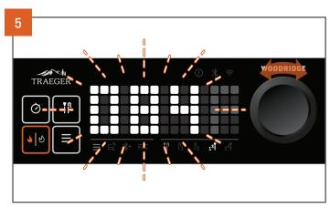
After pressing the selection dial, the numbers on screen will flash, indicating you are in the selection mode. Turn the selection dial to your desired internal goal temperature.
