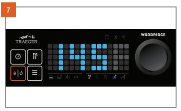
The goal temperature on screen will turn blue when the selection has been confirmed. After confirming this goal, the display will now alternate between showing the goal temperature (in blue) and the current probe temperature (in white) when this probe is highlighted. This probe icon in the probe menu bar turns to blue to indicate that a goal has been set. The controller will alert you when you have reached your target temperature.
