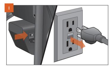
Press the main power switch to OFF (0) and disconnect the power cord. If the grill is still hot, allow it to cool completely.
