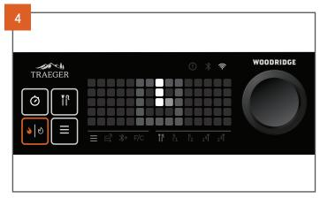
A timer animation will play on screen to indicate that the timer was successfully set. The timer LED button will stay lit up while a timer is set. With timer button selected, the remaining time will display on the screen. Once the remaining time is under an hour, the display will switch from showing "hours: minutes" to "minutes: seconds."
