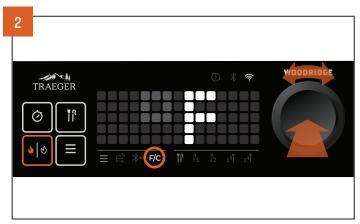
Turn the selection dial until the "F/C" icon is lit in the menu bar. Press the dial to enter the selection mode.
