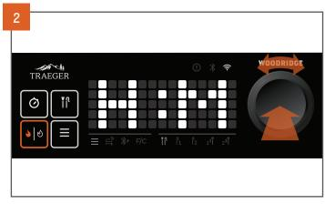
H and M will flash briefly, indicating that you can set hours on the left and minutes on the right. Hours will flash first. Turn the selection dial to your desired hours, then press the dial to lock in hours. If you do not wish to set any hours, press the selection dial when the screen displays 00:00.
