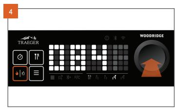
When the desired probe is highlighted in the probe menu bar, (in this example, Bluetooth® probe I), press the selection dial to select it.
