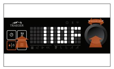
**EDITING:** If you'd like to edit a current probe goal alarm, simply tap the probe button, turn the selection dial to highlight your desired probe in the probe menu bar, and press the dial. Turn the selection dial to the desired temperature and press to lock in your setting.
