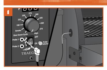
Insert I or 2 meat probes into the probe jacks on the lower left corner of the controller, then thread probes through the access hole grommet on the left side of the grill body.
