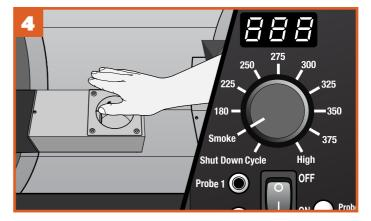
Check that there is air movement from the draft inducer fan by placing your fingers over the firepot. If the hot rod is getting hot, it will turn red.
