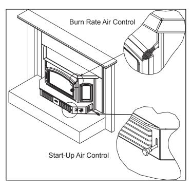
Figure 10.1 Start-up and Burn Rate Air Controls
