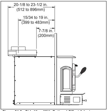
Figure 31.3 - Side View With Optional Offset Adapter
