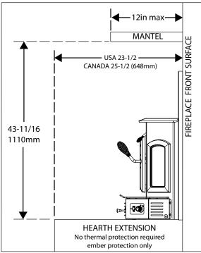
In Canada a full length 6 inch (152mm) S635 flue liner required as per ULC S628. In USA a minimum 5 ft length (1.82m), 6 inch (152mm) diameter flue liner is required as per UL 1482.
