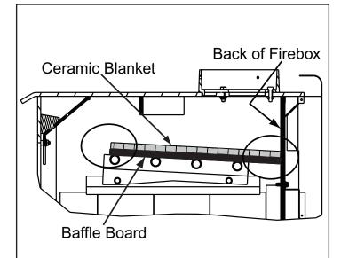
Ceramic Blanket and Baffle Board MUST be in contact with the back of the firebox and even with each other in the front.
