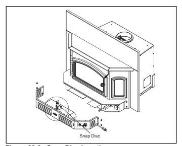
Figure 23.2 Snap Disc Location
