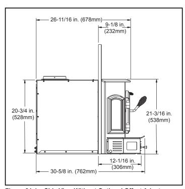
Figure 31.4 - Side View Without Optional Offset Adapter
