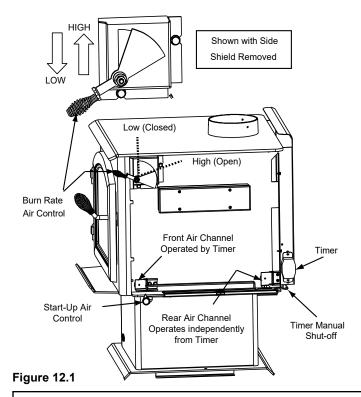
After activating the timer (ACC), if the control is placed within the rear air section on the label it will allow rear air to enter the firebox. This will not interfere with the timer gradually closing the front air channel in 25 minutes. If control is set on "HI" it over-rides the timer (ACC).
