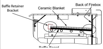
Ceramic Blanket and Baffle Board MUST be in contact with the back of the firebox and even with each other in the front.
