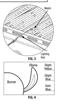
9. After lighting, observe the burner flame. Make sure all burner ports are lit and flame height matches illustration (Fig. 4).
