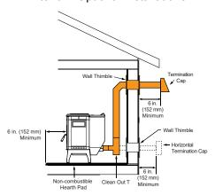
NOTE: In Canada when using a factory-built chimney it must be safety listed, Type UL103 HT (21000F) CLASS "A" or conforming to CAN/ULC-S629M, STANDARD FOR 650°C FACTORY-BUILT CHIMNEYS.
