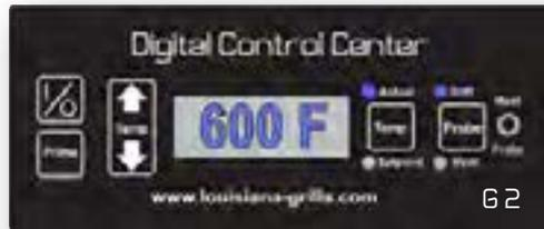
**TIP !** All our digital controls and probes do have a manufacturer +/- tolerance. It is normal for the temperature readings to be off by a few degrees.
