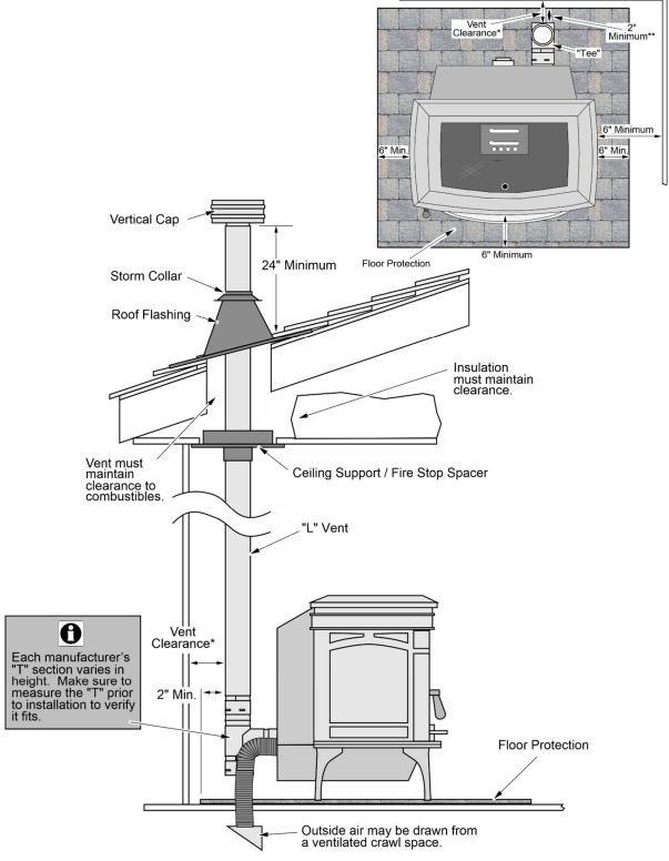
\* Install vent at clearance specified by the vent manufacturer.
