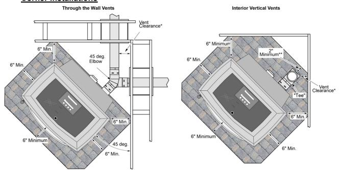
\* Install the vent at the clearance specified by the vent manufacturer.
