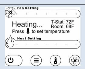
After the stove has successfully ignited the readout will switch from "Starting..." to "Heating..."
