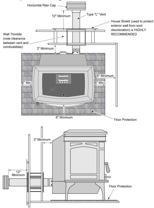
NOTE: Travis Industries recommends a minimum vertical vent of 5' to ensure adequate draft during a power outage.
