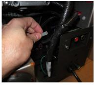
2. Remove the ash pan and the exhaust cover plate. Locate the pressure switch nipple and make sure there is no debris in the opening (use a brush to clean – do not use a vacuum cleaner). Return the stove to its proper configuration.
