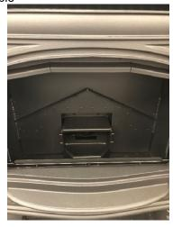
8. With the liners removed, clean all fly ash and debris from the firebox. Clean the liners before replacing them. Make sure to clean the heat exchanger on the firebox ceiling.
