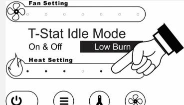
Press the lights on the Heat Setting slider underneath the desired selection (On & Off or Low Burn).
