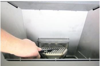
4. Brush away flyash around the burn platform using the brush included with the stove. The flyash will fall into the ashpan below.
