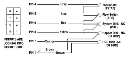
NOTE: text in parenthesis match power control board printed characters
