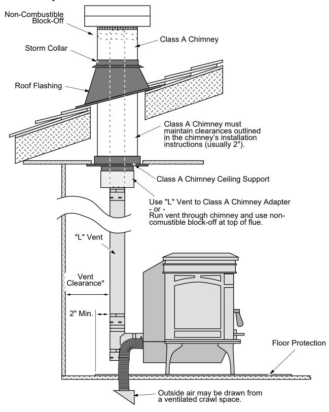
\* Install vent at clearance specified by the vent manufacturer.
