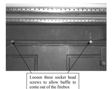
Рното #2 The removable baffle assembly inside the Clydesdale firebox. (Shown looking straight into the firebox through the front door.) DO NOT REMOVE from the firebox unless required (see note in step one).
