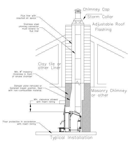
Figure 6 Connecting to a chimney
