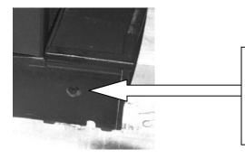
**PHOTO #3** Side view of the ash lip showing phillips screw that must be loosened to remove the ash lip
