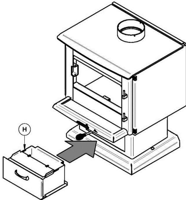
6- Gently flip the stove back on its pedestal making sure not to put too much weight on the rear edge of the base.
