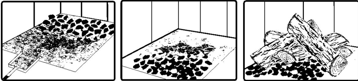
*Remove ash first, and then rake charcoal towards the front of the firebox before loading so that it will ignite the new load.*
