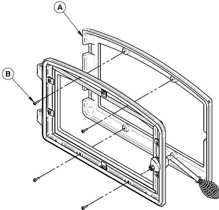
Position the overlay (A) on the door frame and secure it from the inside of the door using the 4 included screws (B).
