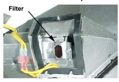
CAUTION: If the filter is not reinstalled, refractive light in the room may result in a fault, thus shutting down of the unit.
