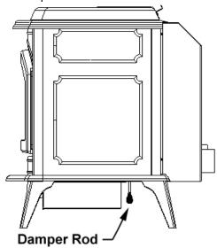
2. Screw damper rod into threaded hole.
