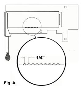
For initial setup, push the damper all the way in (when facing the front of the stove, "in" is to the left, and "out" is to the right) and slowly pull back three notches (see Fig. B).
