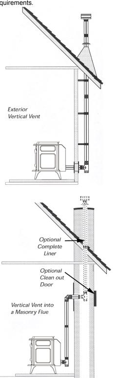
Preferred Installation - Vertical Vent Through the Roof. This venting configuration allows for the best stove performance. The vertical pipe promotes natural draft and with the chimney inside the dwelling, the flue gases stay warm, thus rising at a consistent rate.
