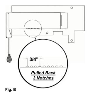
This setting should provide an adequate air to fuel ratio for most installations.
