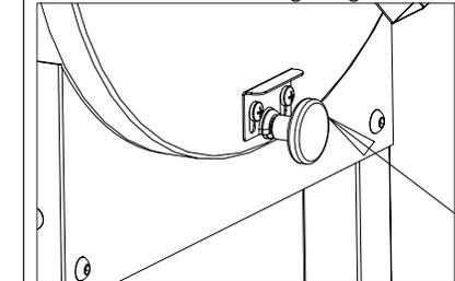
Never open the burner clean-out port when the grill is hot.
