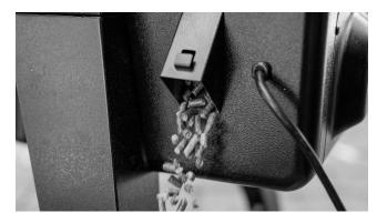
Empty the pellet hopper to prevent your pellets from getting wet or coming into contact with cleaning substances.
