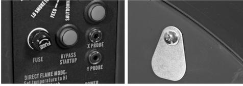
the front panel. If the fuse is blown replace only with 4.0 Amp 125V 5x20mm Fast Blow Fuse. Typical fuse marking will be 4A125V, F4A125V, 4A250V, or F4A250V. Make sure to confirm they are a Fast Blow Fuse. Actual fuse dimensions are 5.2x20mm.
