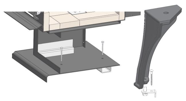
In mobile home installations, the stove must be securely fastened to the floor using the tie-downs provided in the Outside Air kit. (For the pedestal model, remove the ash drawer to access the screw down holes. For the Leg model, use the Leg Anchor Kit (P/N ZR8039) to secure stove to floor.)
