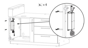
**STEP 06** With the help of another person, direct the regulator hose and electric wires through the cabinet hole and place the griddle body on top of the cabinet.
