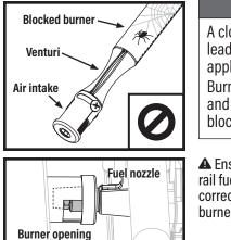
A clogged burner can lead to a fire beneath the appliance. Burner should be removed and cleaned whenever blockages are found.
