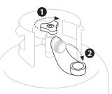
**STEP 02** Hold the regulator in a straight line with the Type 1 valve outlet so as not to cross thread the connection.
