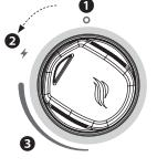
**Note:** If the magnet in the knob is disconnected, the indicator light will be orange. If the knob arrow is facing UP, gas is not flowing.
