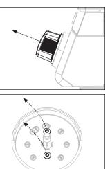
STEP 02 Use a Philips head screwdriver to remove the two (2) M4x10 screws from the knob bezel and set aside.
