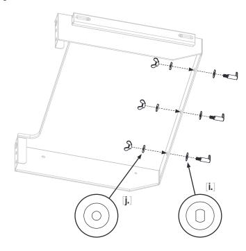
STEP 07 Loosen the two (2) M6x12 bolts on the left side of the griddle body.
