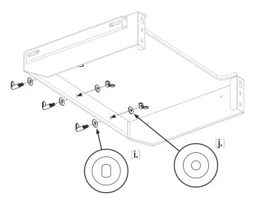
**STEP 06** Use three (3) wing nuts [e.], three (3) washers [i.], and three (3) slotted washers [i.] to attach three (3) shelf pegs [f.] to the right side shelf.
