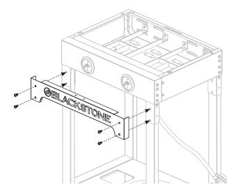
**STEP 07** Use four (4) M6x12 screws [**b.**] to secure the griddle body to the left and right leg assemblies. (**Note:** loosely install these screws, then tighten all M6x12 screws [b.] screws from the previous steps.)
