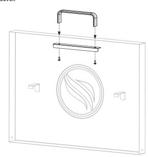
**STEP 14** Hang the hardcover on the back of the griddle top when in use.
