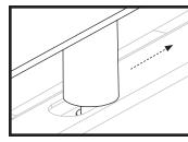
STEP 12 Hang the grease cup in the slot on the back of the griddle body.
