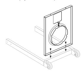
STEP 04 With the help of another person, use two (2) M6x12 screws [b.] to attach the left side of the cart base to the left leg assembly. (Note: DO NOT fully tighten these screws yet.)
