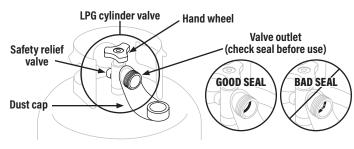
The seal on the valve outlet could, over time, show marked and visible damage or deterioration that might cause a leak even with the connection tightened.
