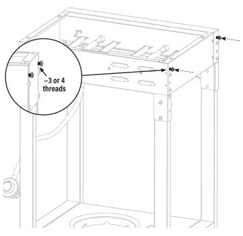
$\underline{\textbf{STEP 10}}$  Hook the side shelf on the top screws on the left side of the griddle body. Use two (2) M6x12 screws [b.] to secure the side shelf to the griddle body. (Note: tighten all four screws.)
