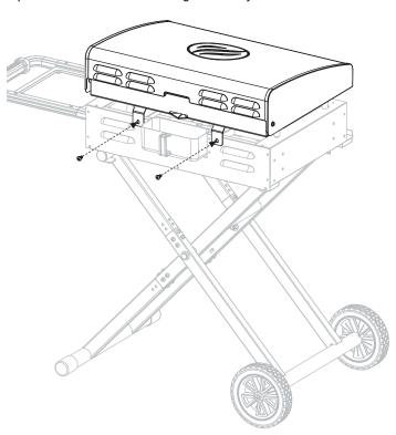
$\underline{\text{STEP 12}}$  Use two (2) M6x16 screws (found within the hood handle) to attach the hood handle to the hood.
