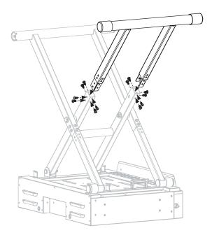
**STEP 05** Use two (2) M10x17 step bolts and bolt sleeves [**b**.] to install the two (2) wheels to the wheeled leg assembly crossbar.
