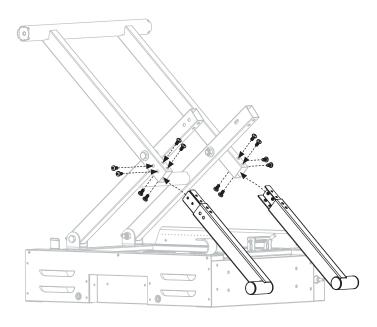
**STEP 04** Set the upper legs in the C clamps. Use twelve (12) M6x12 bolts [a.] to install the lower leg assembly onto the pivoting leg assembly.
