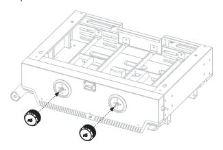
**STEP 02** Turn the griddle body upside down, and pull the locking pin to unlock the legs.
