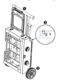
**STEP 08** Lift the side shelf handle and, while putting weight on the lower leg assembly crossbar, pull the griddle up and toward you until the top of the wheeled leg assembly aligns with the C clamps.
