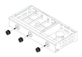
**STEP 02** Screw the four (4) feet into the bottom of the body.
