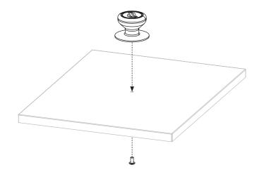
**STEP 07** Place the side burner grate over the round burner. Place the hard cover in place when the burner is not in use.
