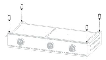
**STEP 03** Set the body on its feet. Use eight (8) M6x12 bolts  $[\mathbf{b.}]$  to attach the two (2) side handles to the side of the body.
