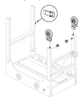
$\underline{\textbf{STEP 02}}$  Use one (1) large thumb screw  $[\boldsymbol{g.}]$  to attach the stabilizing shelf to the right leg assembly.
