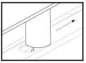
**STEP 10** Remove the two (2) screws pre-installed in the hard cover handles.
