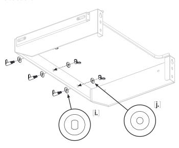
**STEP 05** Use three (3) wing nuts [e.], three (3) washers [j.], and three (3) slotted washers [i.] to attach three (3) shelf pegs [f.] to the right side shelf.
