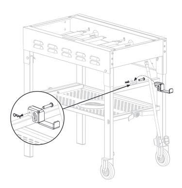
**STEP 04** Use three (3) wing nuts [e.], three (3) washers [j.], and three (3) slotted washers [i.] to attach three (3) shelf pegs [f.] to the left side shelf.
