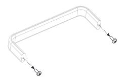
**STEP 11** Use the screws pre-installed in the hard cover handles to attach the two (2) hard cover handles and two (2) hard cover hooks to the hard cover.
