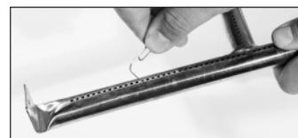
**STEP 06** Carefully replace burners and reattach, with attention to the location of the ignition needle.
