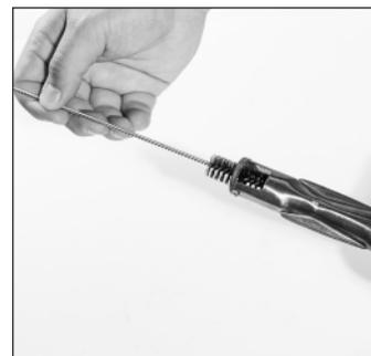
**STEP 04** Brush entire outer surface of burner to remove grime.
