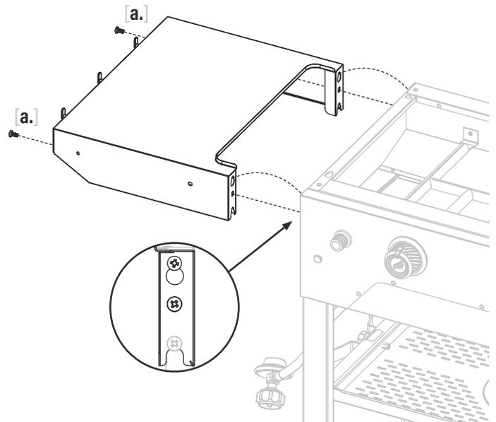
**STEP 07** Use four (4) M6x12 bolts [a.] to attach the side handle to the right side of the griddle body.
