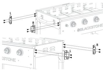
**STEP 08** Thread two (2) M6 step bolts [d.] into the upper holes of the right side shelf.
