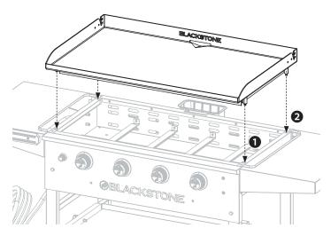
1 Place the two front pins into the front locking holes and push the griddle top back.
