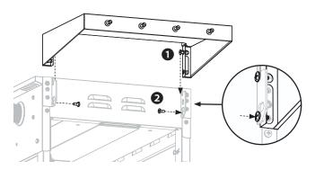
**STEP 11** With the help of another person, place the griddle top onto the griddle body by aligning the four foot pins to the holes on top of the unit.
