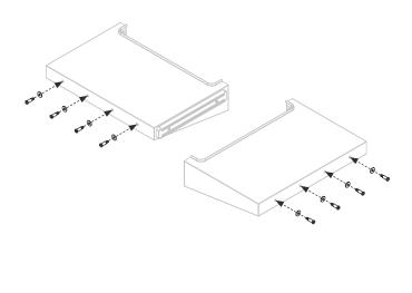
$\underline{\textbf{STEP 10}}$  Thread two (2) M6 step bolts [a.] into the upper holes of the right side shelf.
