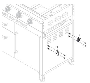
$\underline{\textbf{STEP 06}}$  Thread two (2) M4 step bolts [e.] into the bottom holes of the garbage bag holder brackets.
