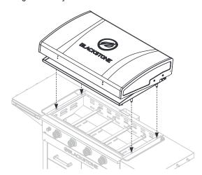
Make sure the front pins are seated in the holes, then push the griddle top back.
