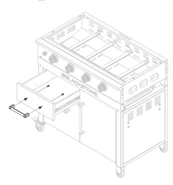
**STEP 05** Use four (4) M6x12 bolts [h.] to attach the garbage bag holder bracket (L) and right garbage bag holder bracket (R) to the right side of the griddle body.
