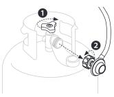
Place dust cap on cylinder valve outlet whenever the cylinder is not in use. Only install the type of dust cap on the cylinder valve outlet that is provided with the cylinder valve. Other types of caps or plugs may result in leakage of propane.
