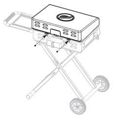
Ensure that all four pins are seated in the holes, then push the griddle top forward to lock the griddle in place.
