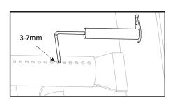
Ensure that the ignition needle is positioned 3-7mm away from the burner tube, positioned above a burner hole.
