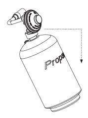
If frosting persists after bottle is angled correctly: Turn off the appliance and disconnect LPG bottle immediately. This indicates a problem with the bottle and it should not be used on any product. Return bottle to supplier.
