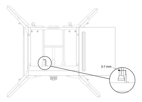
**STEP 08** Place the griddle top and hood on the griddle body by aligning the 4 pins to the holes of the body. Ensure that the pins are fully seated in the holes, then push the griddle top and hood back to lock the griddle in place.
