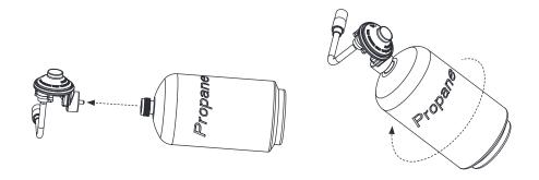
**STEP 12** Insert the gas regulator into the gas line of the griddle. Turn the collar of the gas regulator clockwise to secure it to the gas line.
