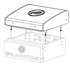
**STEP 02** Place the griddle body upside down on a flat surface. Then, remove the eight (8) M6x12 bolts on the griddle body and set aside.
