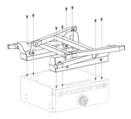
**STEP 04** Open the stand legs. (When the legs are fully opened, the locking pins will engage. To close the legs, pull the locking pins.)
