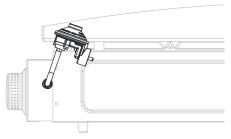
**PLEASE NOTE:** The gas regulator is intended be used at an angle towards the rear of the appliance as shown above.
