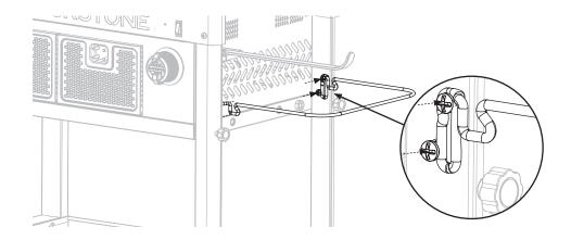
**STEP 10** Use one (1) M6x12 screw (**g**) to attach the propane tank holder to the bottom of the left leg assembly.
