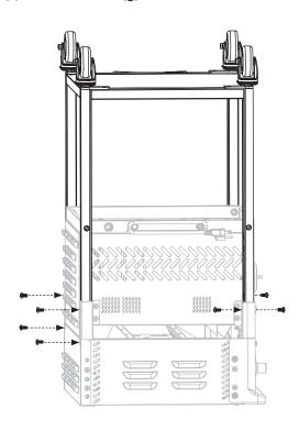
$\underline{\textbf{STEP 04}}$  Use four (4) thumbscrews ( $\mathbf{k}$ ) to secure the legs to the airfryer body.
