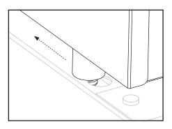
Ensure that the front pins are seated in the holes, then push the griddle top back to lock the griddle in place.
