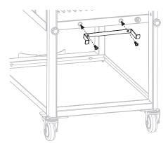
**STEP 13** Use three (3) M6x8 screws (**b**) to attach the three (3) side shelf hooks to the left side shelf.
