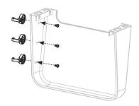
**STEP 14** Thread two (2) M6 step bolts (**c**) into the top holes of the left side shelf. Repeat with the right side shelf.
