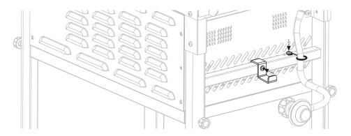
**STEP 12** Use two (2) M6x12 screws (**g**) to attach the power cord bracket to the right side of the griddle.
