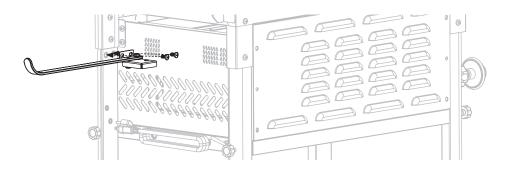
**STEP 09** Use four (4) M4 step bolts (**h**) to attach the garbage bag holder onto the right leg assembly.
