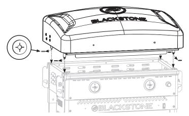
**STEP 07** Use two (2) M6x20 screws (**a**) to attach the hood handle, two (2) hood handle bezels (**j**), and stopper bracket to the griddle hood.
