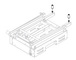
**STEP 02 1** Pull the locking pin to unlock the right leg assembly.
