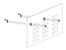
**STEP 08** Use four (4) M5x10 screws to attach the back panel to the rear legs.
