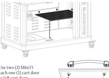
**STEP 16** Use two (2) M6x15 screws to attach one (1) cart door handle to the left cart door.
