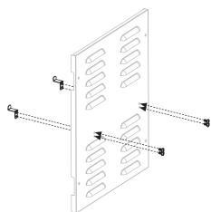
$\underline{\textbf{STEP 14}}$  Use four (4) M5x10 screws to attach the right panel to the right legs.
