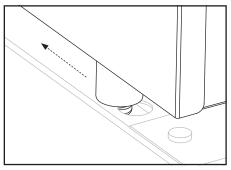
Ensure that all four pins are seated in the holes, then push the griddle top back to lock the griddle in place.
