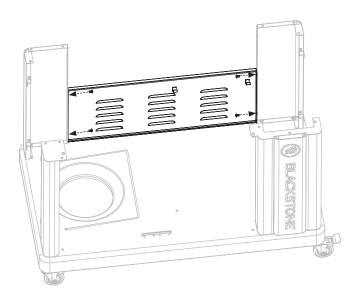
STEP 09 With the help of another person, place the griddle body on the cart and secure with twelve (12) M6x15 screws from underneath the leg plates.
