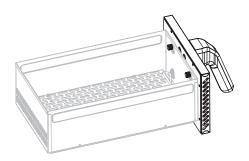
Use the previously removed thumb screws to re-attach the air fryer drawer front panel.
