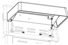
$\underline{\textbf{STEP 24}}$  Use two (2) M5x10 screws to attach the power cord bracket to the back of the air fryer.
