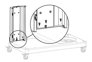
${\bf \underline{STEP~04}}$  Use three (3) M6x15 screws to attach the left-front leg to the cart base.
