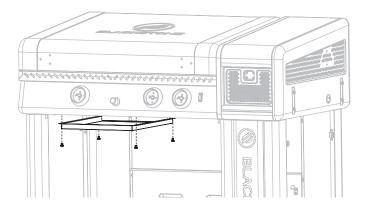
**STEP 11** Use four (4) M6x15 screws to attach the magnet bracket to the lower-front side of the griddle body.
