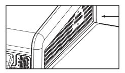
To verify that the air fryer burner has lit, look into the burner chamber from the right side of the unit.
