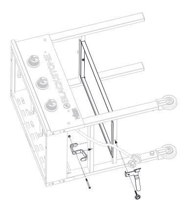
**STEP 04** With the help of another person, set the griddle on its feet. Hang the grease cup in the slot on the back of the griddle body.
