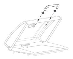
**STEP 10 With the help of another person**, place the griddle top and hood onto the griddle body by aligning the four pins to the holes on top of the unit. Ensure all pins are seated in the holes.
