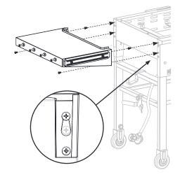
**STEP 09** Use the two (2) M6x16 screws found inside the hood handle to attach the hood handle and handle bezels to the front of the griddle hood.
