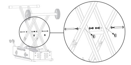
**STEP 10** Use the two (2) removed bolts, four (4) removed washers, two (2) removed nuts and two (2) removed spacers to attach the lower bracket to the leg assemblies.
