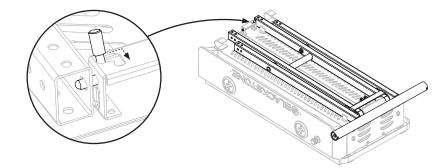
**STEP 05** Raise the legs, and use twelve (12) M6x12 bolts to install the upper legs onto the wheeled leg assembly.
