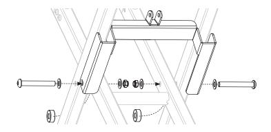
**STEP 11** Use two (2) shear pins and two (2) cotter pins to attach the shock bar to the upper and lower shock brackets.
