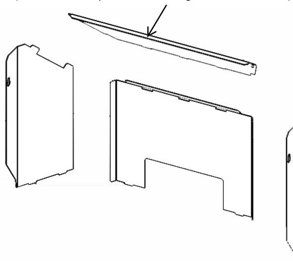
The firebox liners help trap flyash before it enters the exhaust blower. Remove the liners and clean the area behind them following the directions below.
