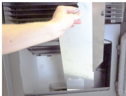
4. Remove the rear liner. Lift it up and remove it from the firebox.
