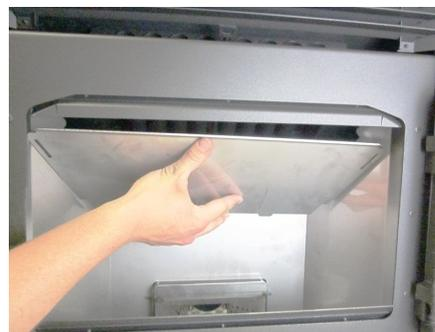
3. Remove the side liners. They have keyhole slots that fit over screws on the side of the firebox. Lift them up, tilt them inwards, then remove.
