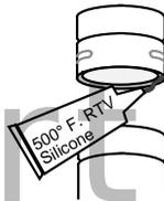
Seal each vent section (including adapters, elbows, etc...) by injecting a liberal amount of 500° F. RTV silicone into the gap between sections.
