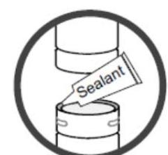
The exhaust system must be completely airtight and properly installed. The pellet vent joints must be sealed with RTV 500° F. (260° C.) silicone sealant.
