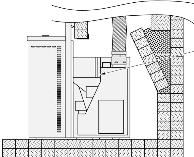
The exhaust quick-connect can be removed to allow for installation and cleaning.
