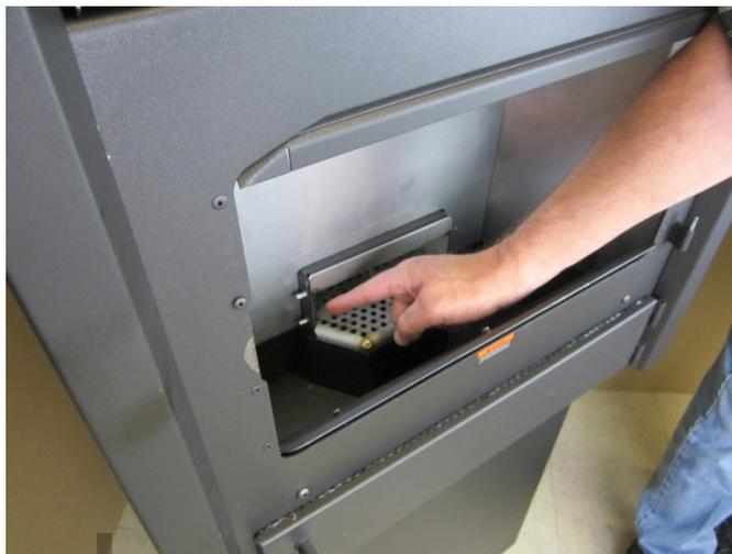
3. Use the cleaning tool to scrape away hardened clinkers or buildup on the fire platform. Use the narrow tip to clear any plugged holes. The fire platform must be free from buildup for the pellets to burn completely.
