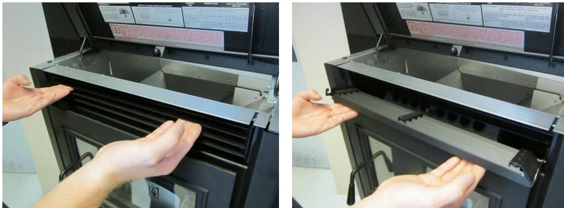
2. Hook the cleaning tool onto the heat exchange scraper rod as shown below.
