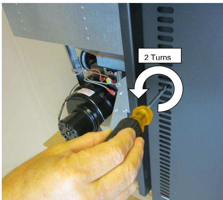
4. Slide each side panel forward and place aside. The side panels have slots that fit over the screws.
