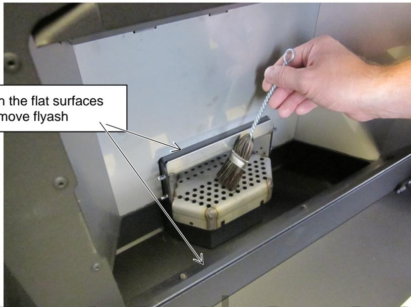
5. Lift the fire platform out of the firebox and remove any flyash below the burn platform.
