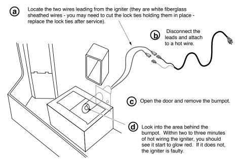
If the igniter does glow red, the igniter is functional. Next, check the wires leading to the igniter.
