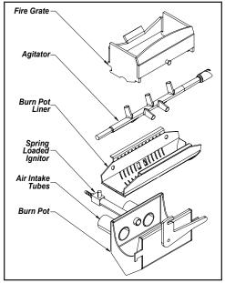
Figure 8: VF-55-FS Burn Pot Assembly.
