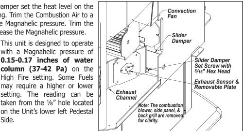
Figure 6: Slider/Damper Plate in Unit.
