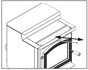
Figure 9: VF-55-FS Heat Exchanger Cleaning.
