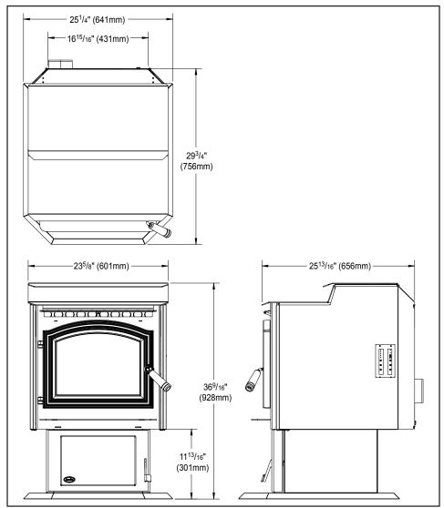
Figure 1: Dimensions of VF-55-FS.
