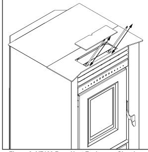
Figure 9: VF100 Burn Heat Exchanger Cleaning.
