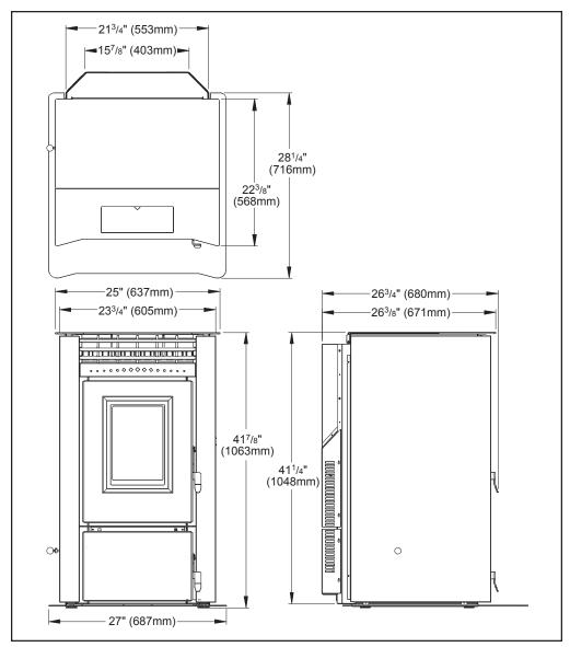
Figure 1: Dimensions of VF100.
