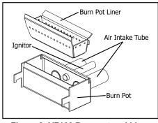
Figure 8: VF100 Burn pot and Liner
