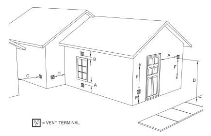
NOTICE: This unit shall be installed in such a way that the exhaust gases are directed so they do not jeopardize people, overheat combustible structures, or enter buildings.
