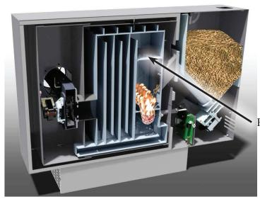
Insure that the flame impingement baffle is installed properly. If the baffle is not installed properly, push the plate up in the void at an angle, rotate it to horizontal and place it on the metal stops.
