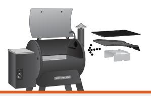
When flames start to come out of the firepot, turn the switch OFF (**0**). Let the grill cool down. Now you're ready to place the heat baffle, grease drain pan, and porcelain-coated grill grate back into the grill.
