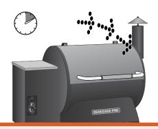
With the door closed, turn the switch ON (I) and the temperature dial to SMOKE. In about 2 minutes, the pellets will ignite and whitish-gray smoke will come out of the grill. After the pellets have ignited, turn the temperature dial to any cooking setting
