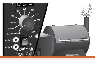
With the door closed, turn the switch ON (I) and the temperature dial to SMOKE. In about 2 minutes, the pellets will ignite and whitish-gray smoke will come out of the grill. After the pellets have ignited, turn the temperature dial to any cooking setting desired.
