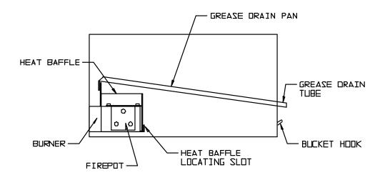
**RECOMMENDATION** for ease of clean-up: Line the Grease Drain Pan (163) with heavy-duty aluminum foil. Be sure the edges and ends of the foil are tight against the bottom of the Grease Drain Pan (163).
