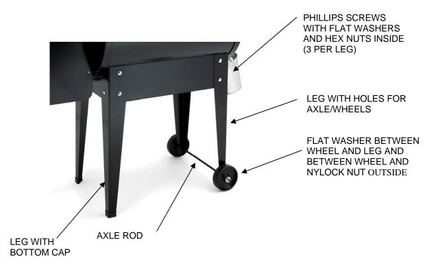
**NOTE:** Install all Leg Screws and Nuts, 3 in each Leg, LEAVING NUTS LOOSE. Set Grill upright to level and then tighten all nuts.
