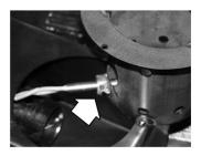
Set the Igniter Down in place, and remove the Igniter wiring by first unplugging it from the controller, carefully remove the plug at the end of the Igniter wire by cutting it off. Carefully work the Igniter wire back thru the unit and remove the entire Igniter from the grill.
