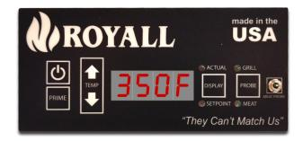
The grill temperature probe setpoint can be adjusted with the UP and DOWN buttons. The grill temperature setpoint defaults to 350 degrees, but can be adjusted between 180 and 500 degrees in 5 degree increments.
