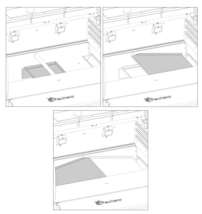
Step 16 (cont'd): Insert Heat Deflector, Drip Pan, Cooking Grates, Meat Hanging Rod, and Drip Bucket
