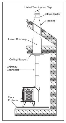
Figure 8.3 Interior Prefabricated Chimney
