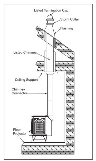
Figure 14.2 - Prefabricated Interior Chimney
