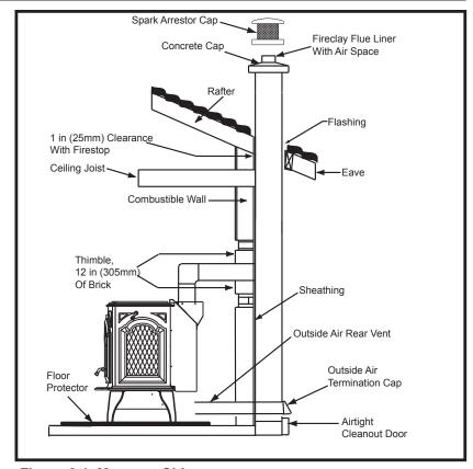
Figure 8.1 Masonry Chimney
