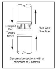
Figure 17.2 Chimney Connector (Stove Pipe)
