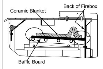
Ceramic Blanket is bunched up at the back of the firebox and NOT even with the Baffle Board in the front.
