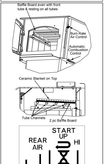
After activating the timer (ACC), if the control is placed within the rear air section on the label it will allow rear air to enter the firebox. This will not interfere with the timer gradually closing the front air channel in 25 minutes. If control is set on "HI" it over-rides the timer (ACC).
