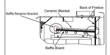
Ceramic Blanket and Baffle Board MUST be in contact with the back of the firebox and even in the front.
